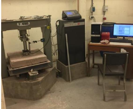
Figura 17- Ensayo de panel EFNARC.
