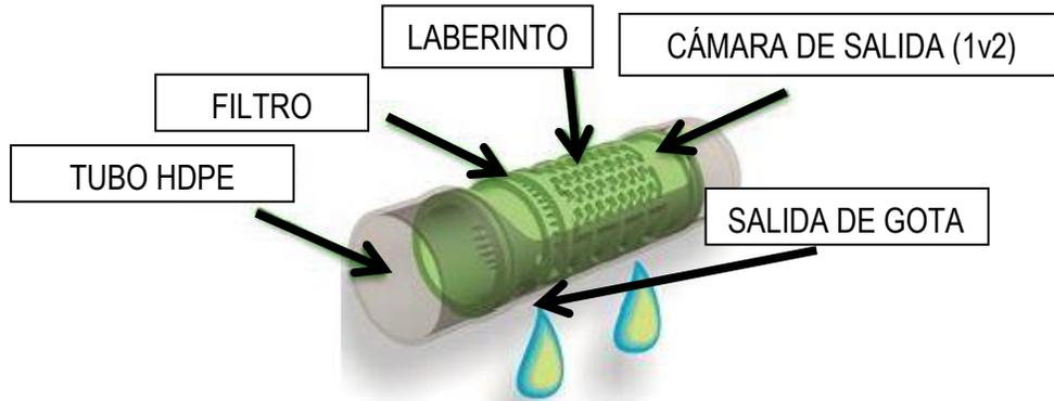
Figura 5.22. Gotero Rivulis Plastro Hydromine 16/35 – 1.6 lph
