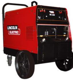
Figura 1-2: Maquina de soldar
