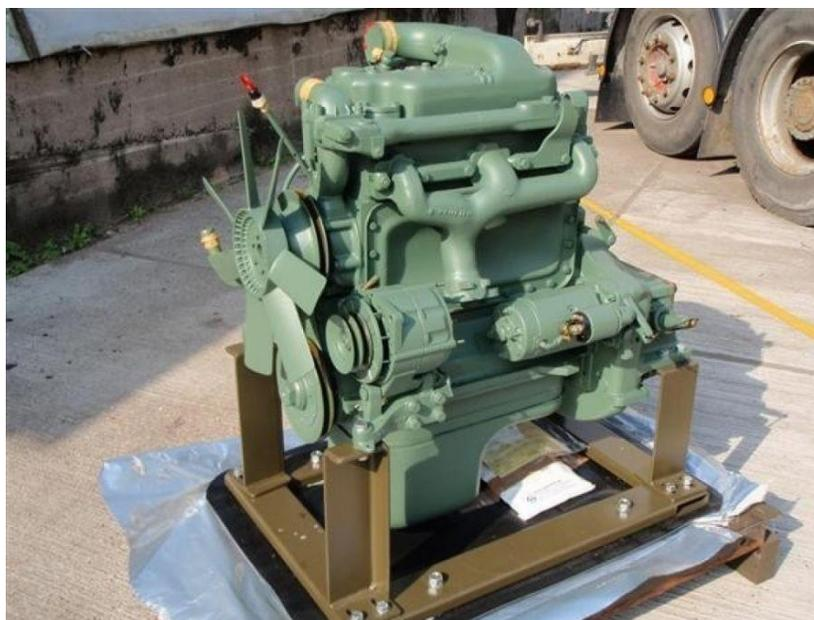
Figura 11: Motor mercedes-benz OM314
