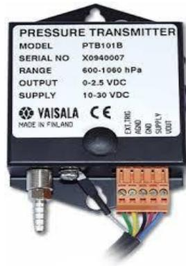
**Figura 1.16:** Pressure transmitter Vaisala, Modelo PTB 101B.-
