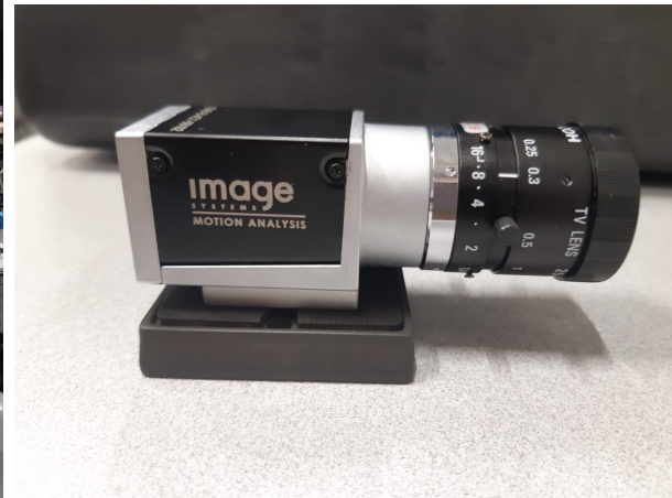
(b) DIC system camera used to take measures with the software TEMA.
