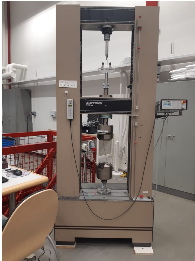
Figure 3.5: Alwetron machine utilized for performing the pre-crack and fatigue toughness test.
