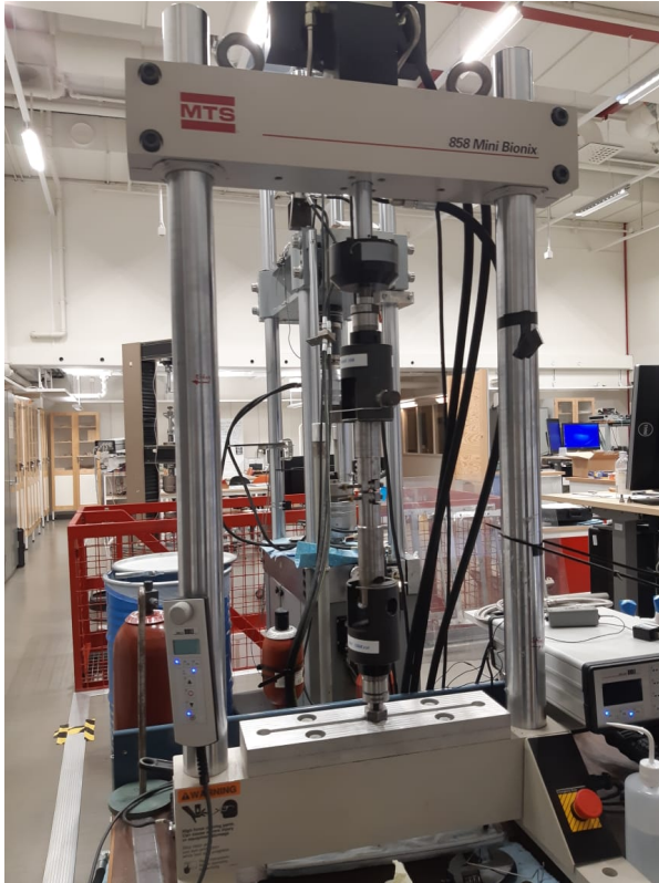
(a) Mini Bionix 858 machine used for the fatigue crack growth rate tests.
