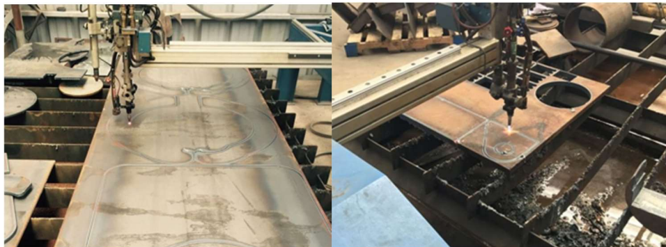
Figura 2.11 Mesa de corte cnc "HNC-2100X" Fuente M&N Mining Figura 2.12 Mesa de corte cnc "HNC-2100X" Fuente M&N Mining
