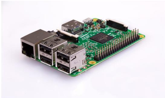
Figura 2.14: Raspberry Pi 3 Modelo B, Fuente: [www.raspberrypi.org](http://www.raspberrypi.org)
