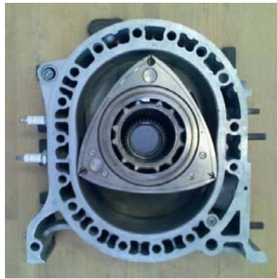
Figura 1.33: Motor Wankel ( Fuente: Embry-Riddle Aeronautical University )
