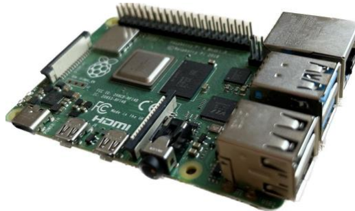
Figura 2-7 Raspberry Pi 4 Model B
