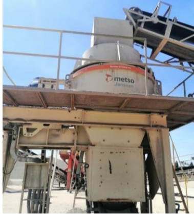
Figura 1-12: Chancador Metso VSI Barmac® B7150SE™
