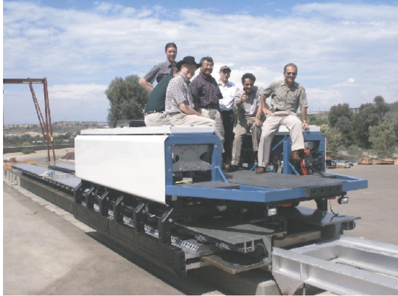
Figura 14: Prueba experimental Inductrack (A. M. G. Jacob et al. [14])
