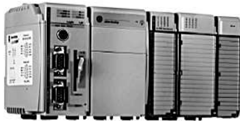
Figura 2.1: PLC Allen-Bradley CompactLogix L35E
