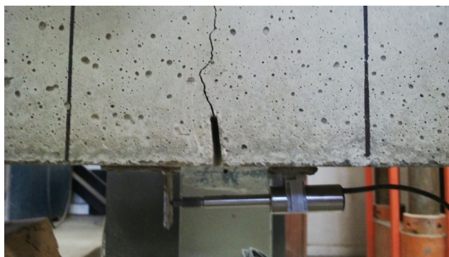
FIG.14: ENTALLA PROBETAS EN14651.
