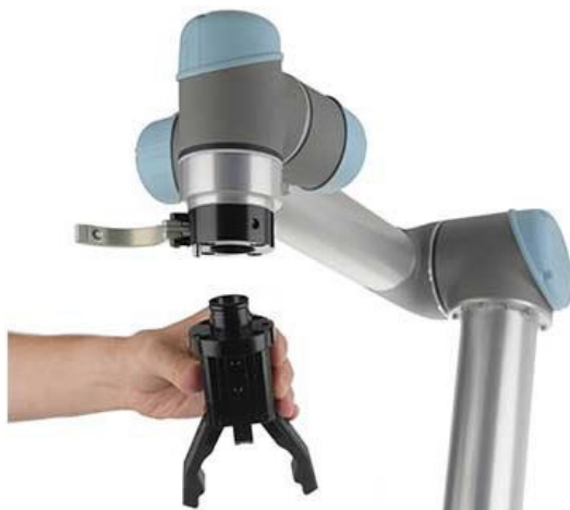
Figura 52: conector SHW de GRIP (Fuente: https://www.grip-gmbh.com/connect/shw )
