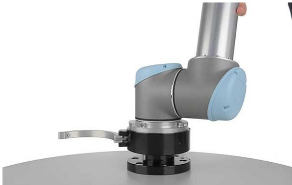
Figura 55: Conector de base GRIP (Fuente: https://www.grip-gmbh.com/products/connect ).
