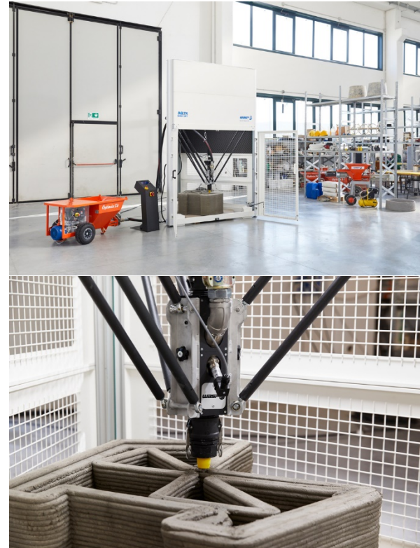
Figura 22: Impresora Delta WASP 3MT CONCRETE (Fuente: https://www.3dwasp.com/en/concrete-3d-printer-delta-wasp-3mt-concrete/ ).
