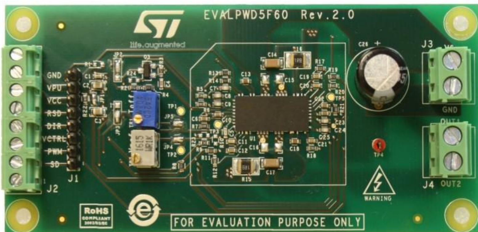
Figura 2.6: Inversor puente H EVALPWD5F60 [19]
