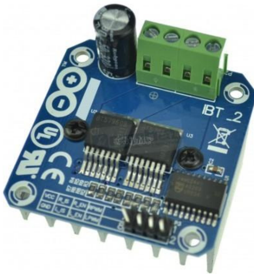
Figura 2.1: Puente H BTS-7960 [14]
