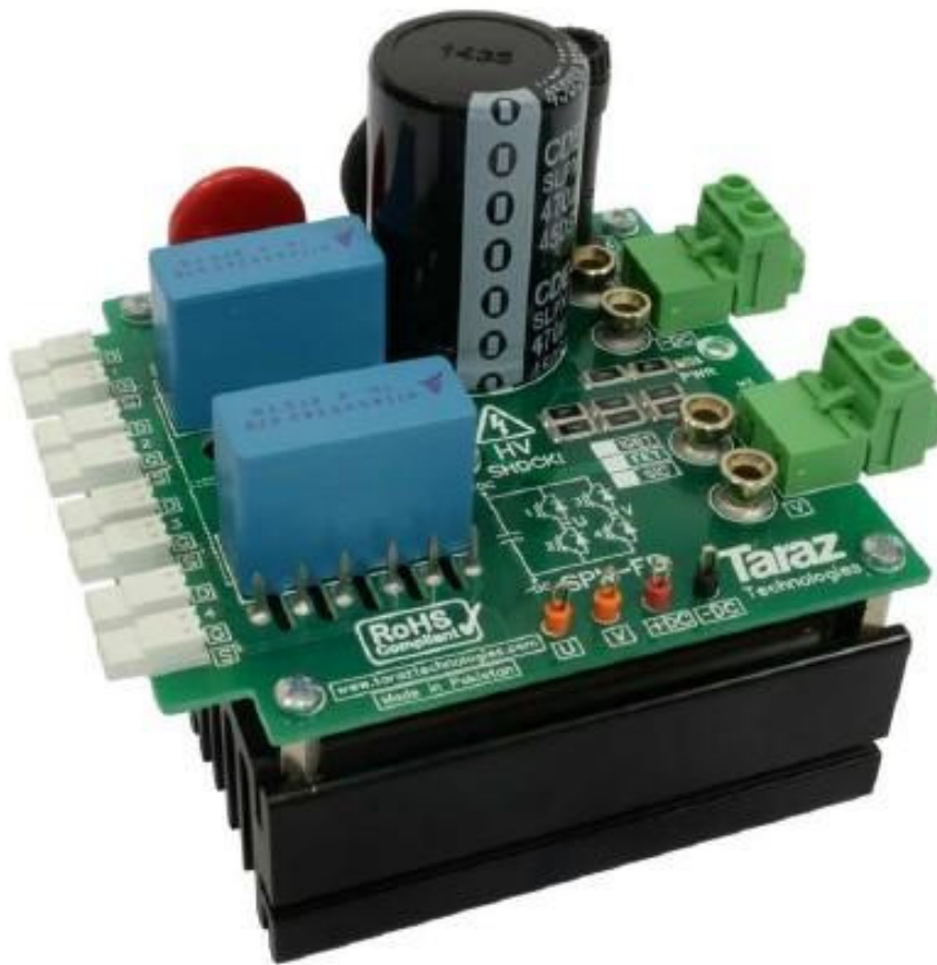
Figura 2.5: Puente H SPM-FB[18]
