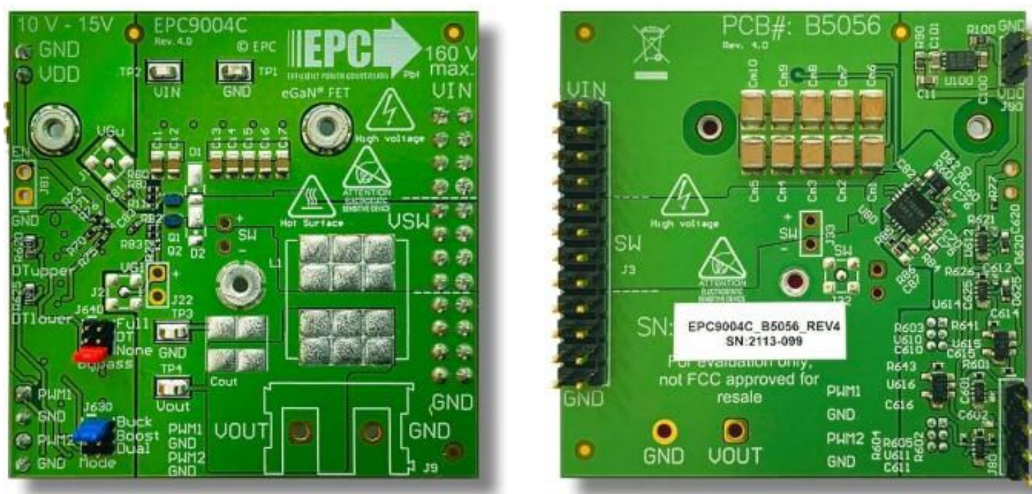
Figura 2.15: Semi puente H EPC9004C [21]
