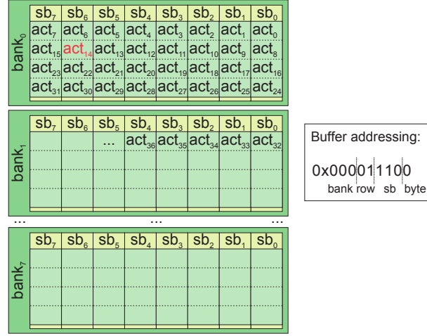
Figure 2.2: Bank organization of a 512-byte I/O buffer and an example of addressing. Label sb refers to sub-bank.
