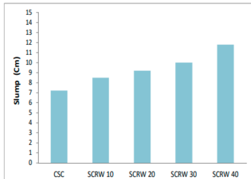
Fig. 11 - Slump of crushed sand concrete as function of rubber waste content. (Mohamed & Djamila, 2018).
