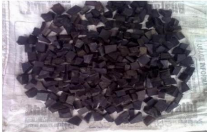
Fig. 5 - Prepared sample of chipped rubber aggregates (Okolnikova et al., 2023)
