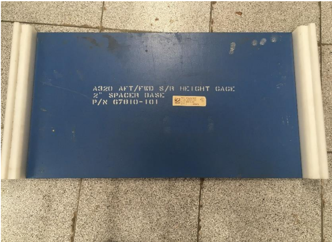
Figura A-15 Spacer base tobogán-balsa AIRBUS 320 fixture.
