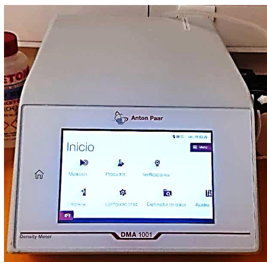
Figura 3-4 Densímetro digital ANTON PAAR DMA1001[30]
