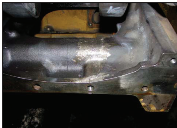
Figure 12 Add Charge Cracked/welded
