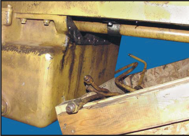
Figure 5 Damaged Core Refund Parts not reassembled to core after dealer inspection
