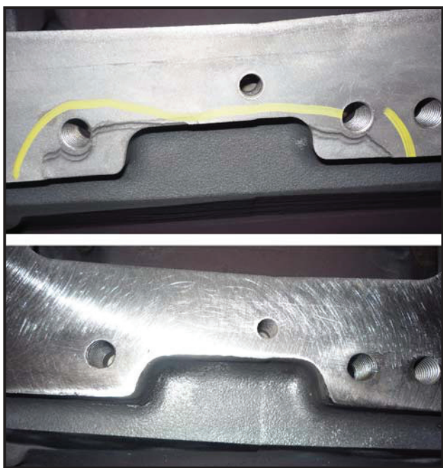
Figure 13 Full Core Refund Cosmetic damage/repair
