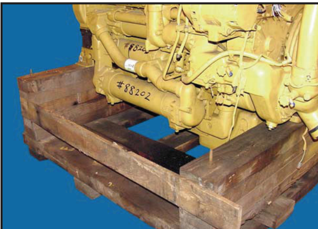
Figure 9 Add Charge Core not returned on correct stand
