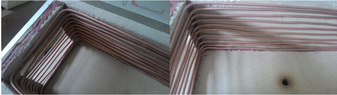
Figure 2.12: Insulation box with the copper pipes system
