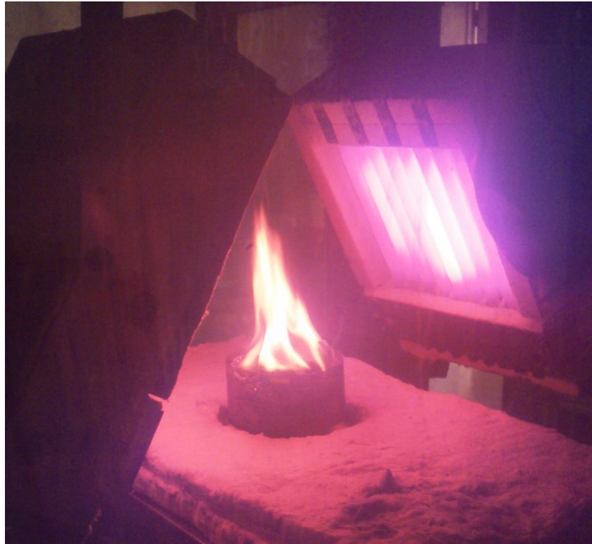
Figure 2.2: Position of the sample in the calorimeter
