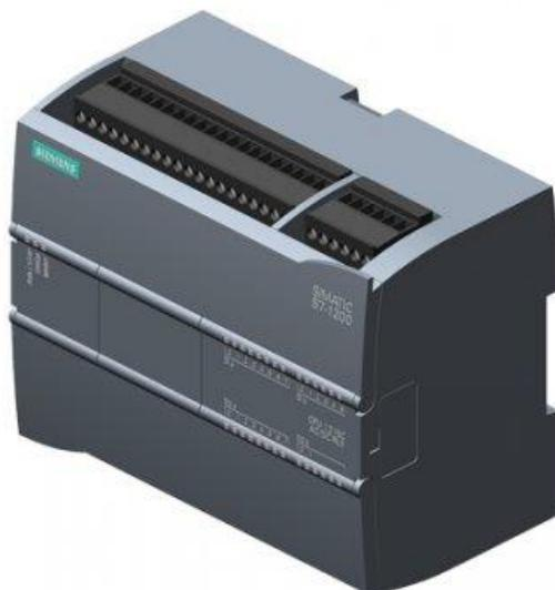
Figura N°5. PLC SIMATIC S7-1200 [5]
