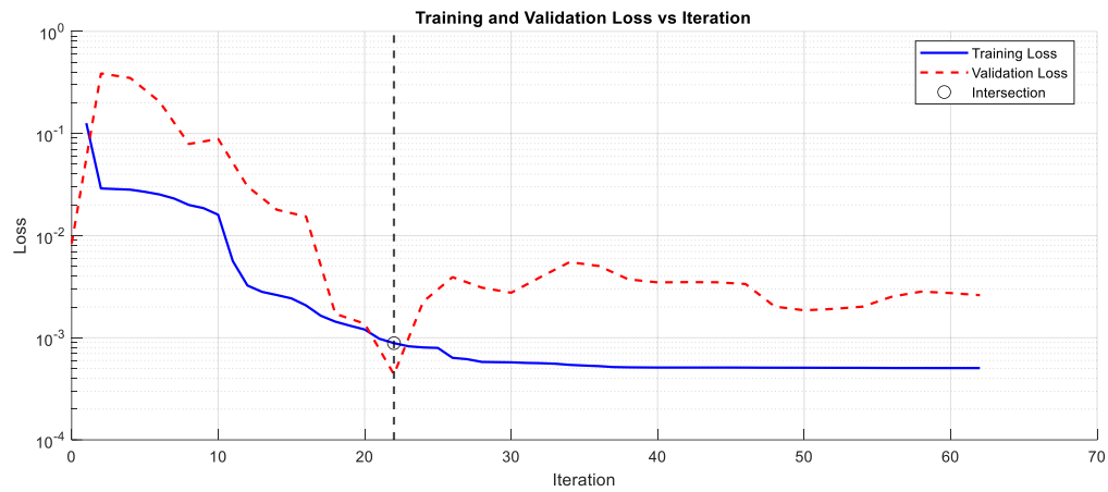
Fig. 124: Training and validation loss vs. iteration for the Hill Model (two-step excitation).
