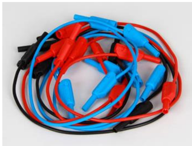
FIGURA 13.6 CABLES TABLERO LEYBOLD 4 MM.
