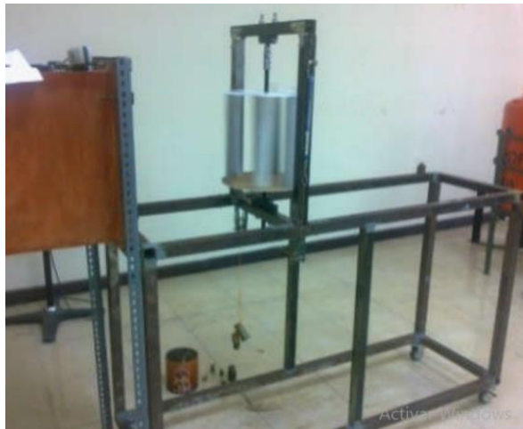
FIGURA 4.14 TURBINA SIN ALABES ORIENTABLES “PERFORMANCE OF COMBINED VERTICAL AXIS WIND TURBINE BLADE BETWEEN AIRFOIL NACA 0018 WITH CURVE BLADE WITH AND WITHOUT GUIDE VANE”.
