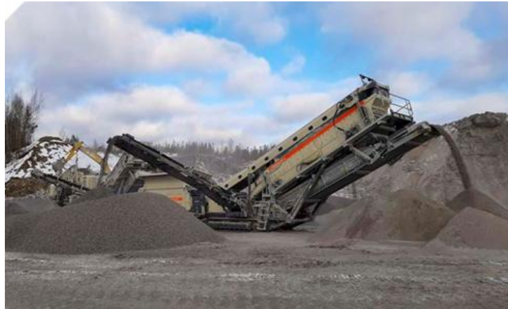
Figura 2.7 " Lokotrack mobile screen"
