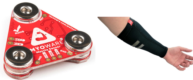
(a) Placa principal del sensor (b) Electrodo seco sugerido Myoware
