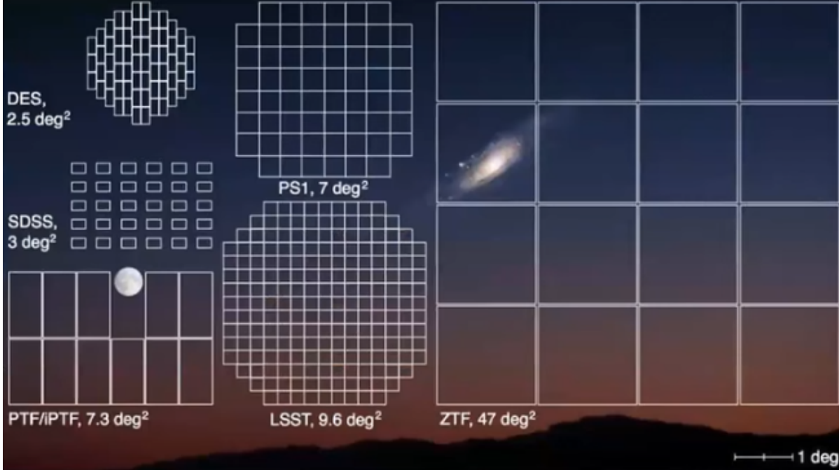
Figure 3.1: Field-of-view of different ongoing and future photometric ground-based surveys, which displays the large sky coverage of ZTF.
