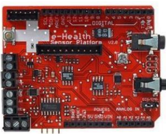
Figura 3: e-Health Sensor Platform for Arduino and Raspberry Pi, https://www.openhacks.com/page/productos/id/1605/title/e-Health-Sensor-Platform-for-Arduino-and-Raspberry-Pi
