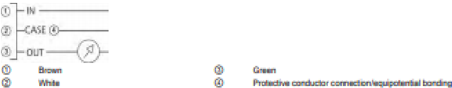
Figure 5-2 Pressure transmitter, electrical connection
