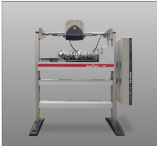
TorsionLine torsion testing machine with testControl II
