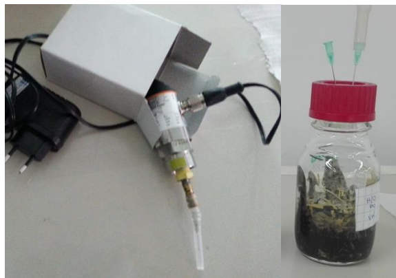
Figure 7. Pressure transducer used (left) and anaerobic digestion assay (right).
