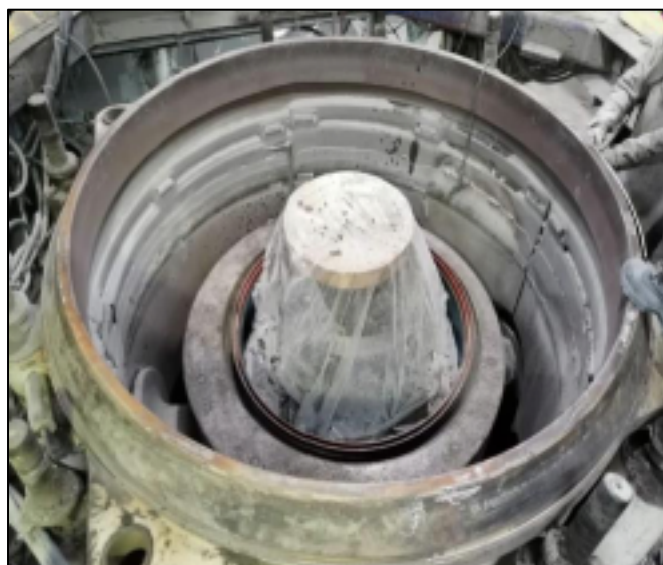
Figura 3-1: Main frame liners T500, (registro personal).
