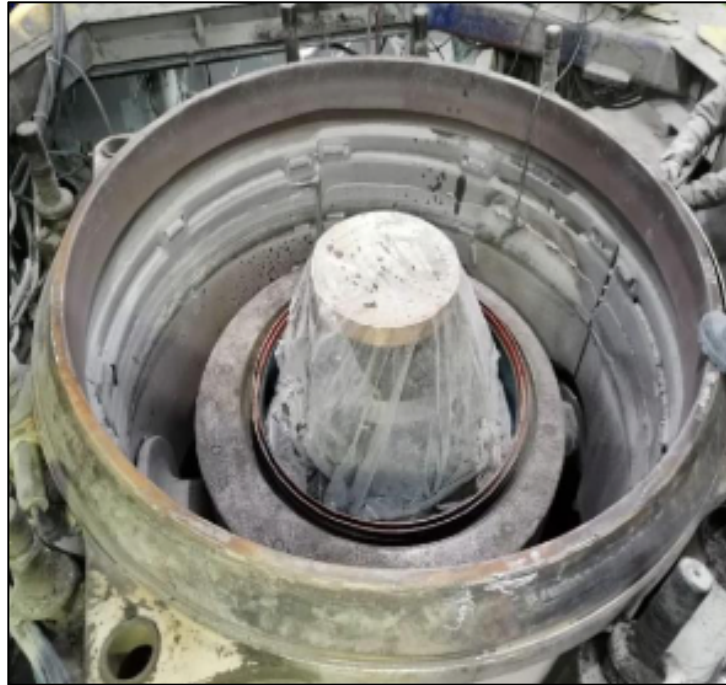
Figura 1-10: Planchas circulares main frame liner. (Registro personal)
