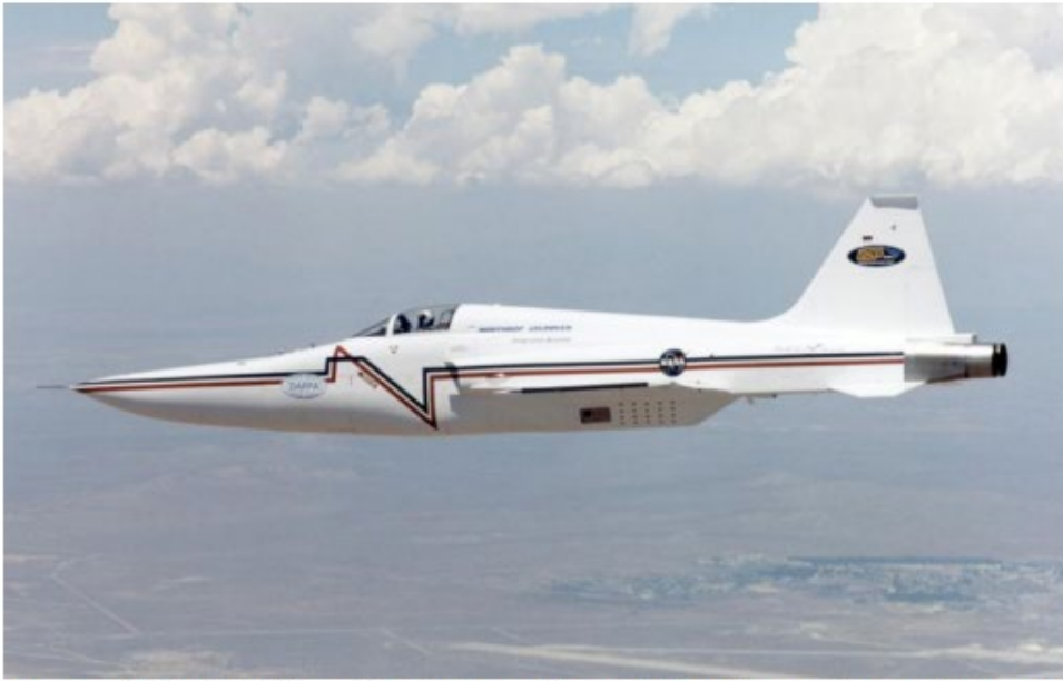
Figure 3. F-5E Tiger II with lengthened fuselage. Demonstrator for the vehicle shaped sonic boom test (NASA Photo)
