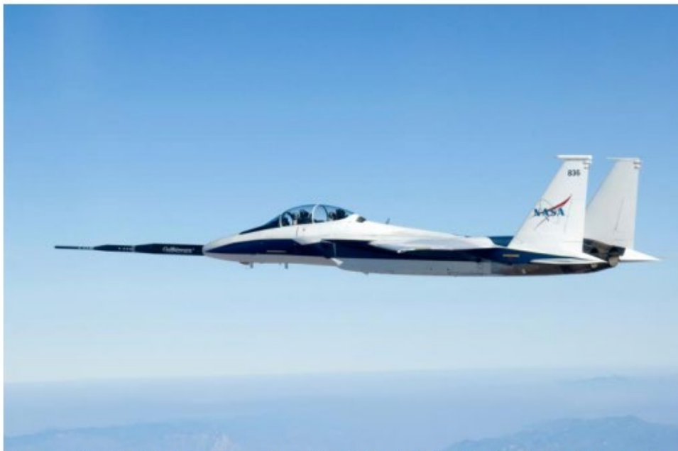
Figure 3. F-15B equipped with "Quiet Spike". A Collaboration between Gulfstream Aerospace and NASA
