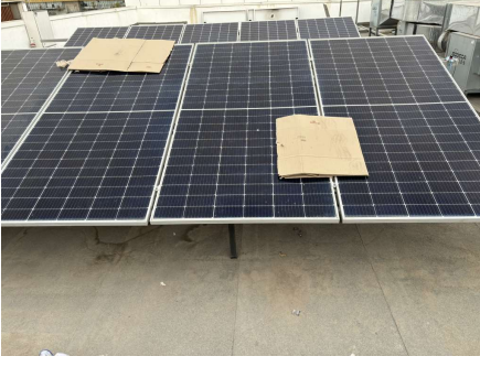
Fig. 5. Experimental photovoltaic array under partial shading.
