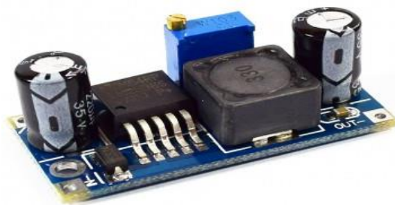
Figura 2-18. Conversor DC-DC LM2596
