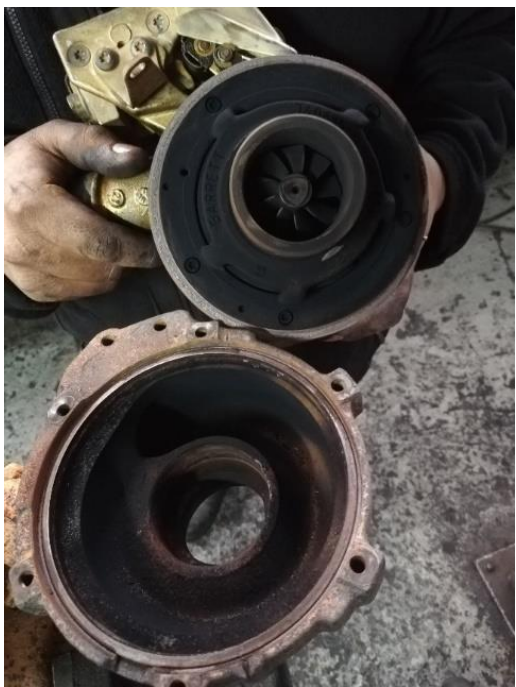
Figura 3-8: Interior carcasa escape
