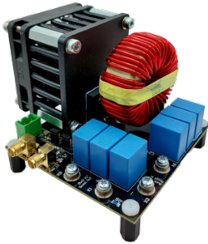
Figura 1.6: Tarjeta NEVB-HB-GAN111-650WSB - Nexperia
