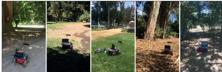
FIGURE 3.4: Several snapshots of the robot driving through the experimental locations. Illumination varied from cloudy to clear sky conditions. (Yandun et al., 2018) © 2018 Elsevier.
