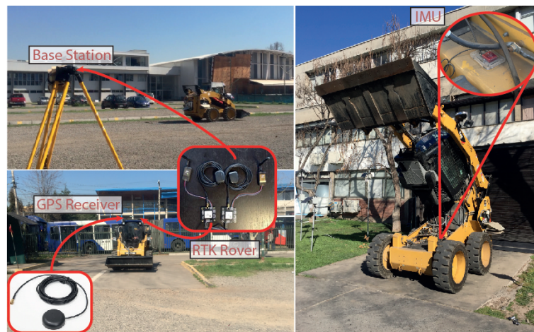
FIGURE 4.18: Sensors employed in experimental tests. The IMU was located in the vehicle body. The GPS and RTK antennas were placed at its top.
