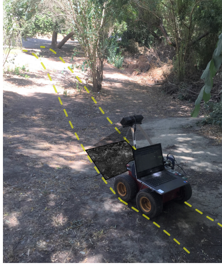
FIGURE 3.3: Experimental setup employed to test the proposed approach using a mobile robot driving through agricultural fields. (Yandun et al., 2018) © 2018 Elsevier.
