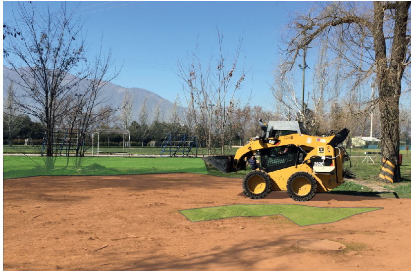
FIGURE 1.8: Earthmoving machine navigating on a typical agricultural off-road scenario. Terrain variability, vehicle characteristics and lack of GPS signal induce uncertainty in movement predictions and slip detection. Robot positioning and wheel slippage can thus be considered as random variables in the navigation process.
