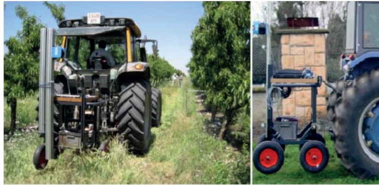
FIGURE 2.2: Two views of the developed scanning system based on the SICK LiDAR. (Auat Cheein et al., 2015) © 2015 Elsevier.
