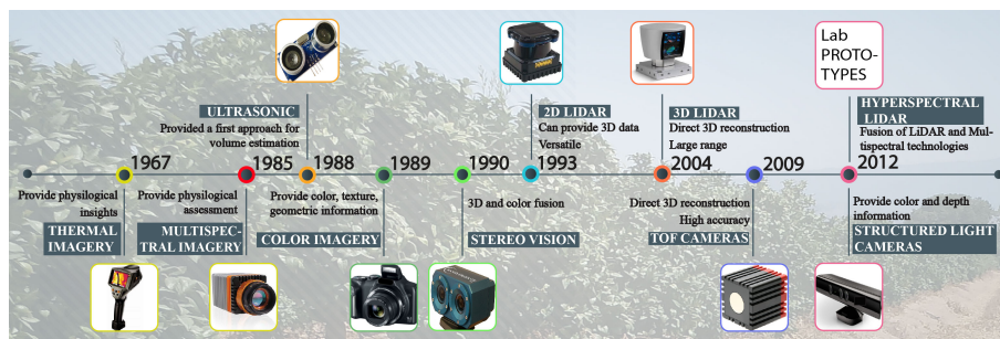
FIGURE 1.7: Evolution in the use of range and artificial vision sensors for morphological characterization and fruit/plant detection. The years report the first use of these sensing systems for agricultural purposes. (Yandun et al., 2017) © 2017 IEEE.
