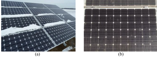
Fig. 2. Long term partial-shading examples. (a) snow accumulation - (b) dust accumulation
