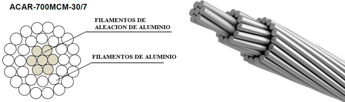
Figura 3.8: Conductor ACAR 700 MCM 30/7
